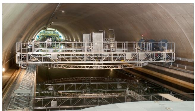
The silent carriage is fitted with a mooring ring so that fixed or moored test subjects can be rotated and exposed to any wave direction. High-speed cameras, LED illumination and optical tracking equipment can also be mounted.
