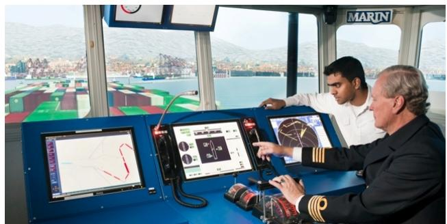
Full Mission Bridge II (FMB II), has a 210 degrees visual projected image. In addition to the projection system, the rear view is presented on three separate displays, thus providing almost 360 degrees view. Additional viewing positions offering a 3D view from any observation point can be installed.
